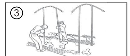
Embedding Arch Pipe
